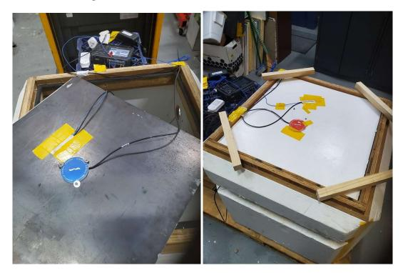
Data Logger with Heat Flux sensors and Temperature probes has been employed for data collection
