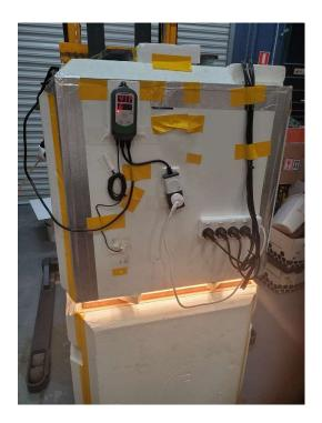
The test chamber is designed to accept substrate samples where top side is fitted with a permanent source of heat (4 x halogen light fittings of 500W each).
