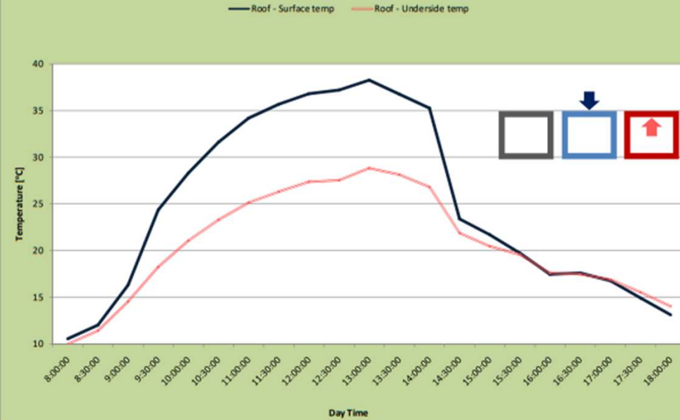
Graph No. 8: Overall reduction of temperature when 0.5mm of C-COAT is applied
