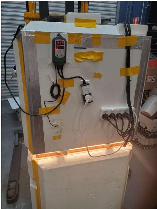
The test chamber is designed to accept substrate samples where top side is fitted with a permanent source of heat (4 x halogen light fittings of 500W each).
