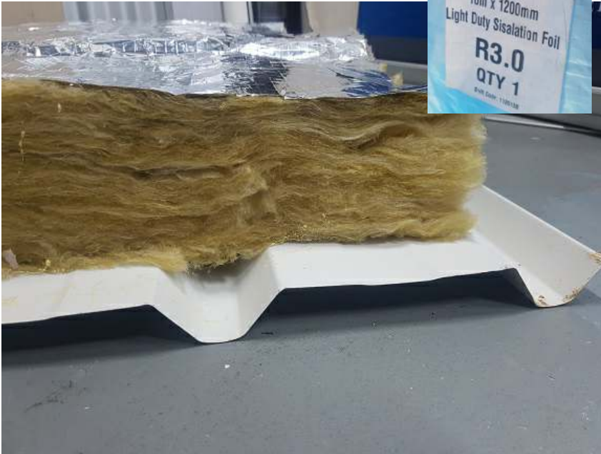
Roof with 130mm classic insulation R3.0 underside
