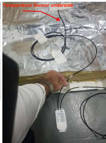
Roof with 130mm insulation R3.0
